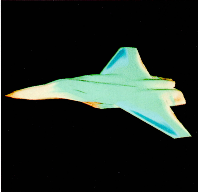
This simulation, which is based on a Navier-Stokes analysis, depicts surface pressure predictions for the F-15 Eagle at Mach 0.9.
