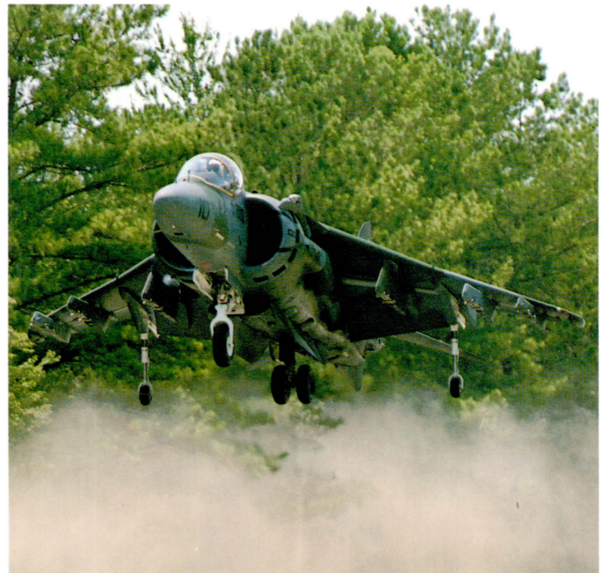
The AV-8B Harrier II can operate from small, unprepared sites and roads close to front lines.
